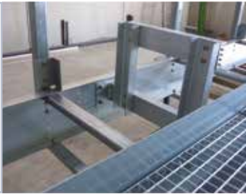
Hot dip galvanized conveyor supports, with adjustable height.
